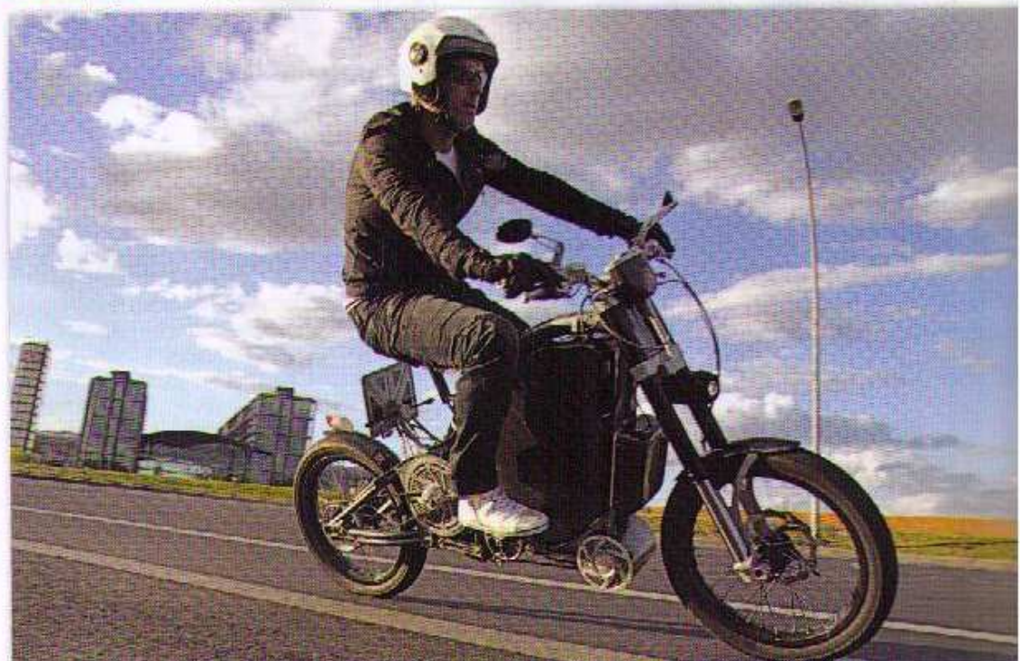
Schizo cycle – The eRockit had to be made out of motorbike parts because bicycle parts just couldn't take the strain
